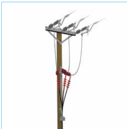
With cable termination
