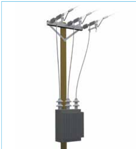
Pole-mounted transformer substation
